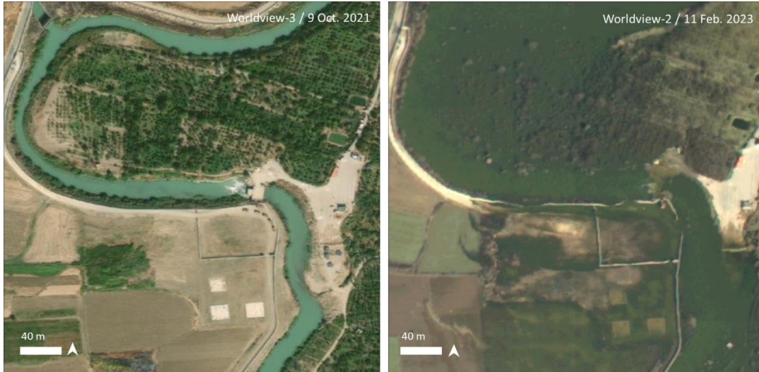
Figure 24. The Orontes River before and after floods. The pre image is acquired by Worldview-3 on the 9 th of October 2021, while the post image is acquired by Worldview-2 on the 11 th of February 2023. The post image shows damage on water infrastructure.
