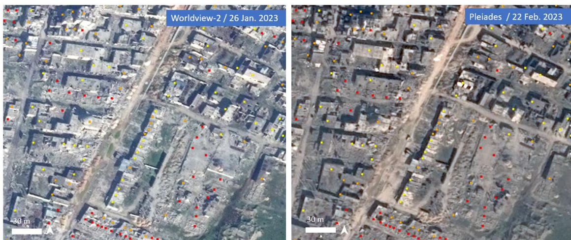
Figure 13. This image shows inset 2 with destroyed, damaged and potentially damaged buildings in southwestern part of the city Aleppo before and after the earthquake of 6 th of February 2023. The pre imagery from the Worldview-2 satellite acquired on the 26 th of January 2023, and the Pleiades satellite acquired on the 22 nd of February 2023 visualise that damage was already existent prior to the earthquake
