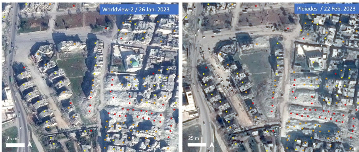
Figure 12. This image shows inset 1 with destroyed, damaged and potentially damaged buildings in southwestern part of the city Aleppo before and after the earthquake of 6 th of February 2023. The pre imagery from the Worldview-2 satellite acquired on the 26 th of January 2023, and the Pleiades satellite acquired on the 22 nd of February 2023 visualise that damage was already existent prior to the earthquake.
